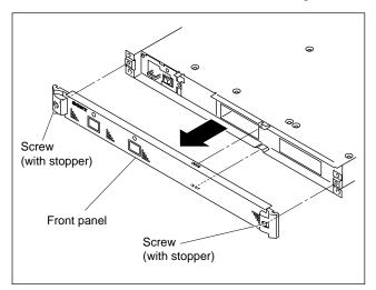
2. Remove the two screws and remove the blank panel in the empty slot for the backup power supply unit.
